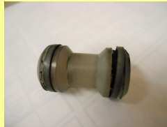
Parts worn out by no lubrication
