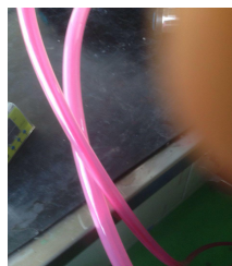
Ink stain dirty remain on hose after solvent circulation washing
